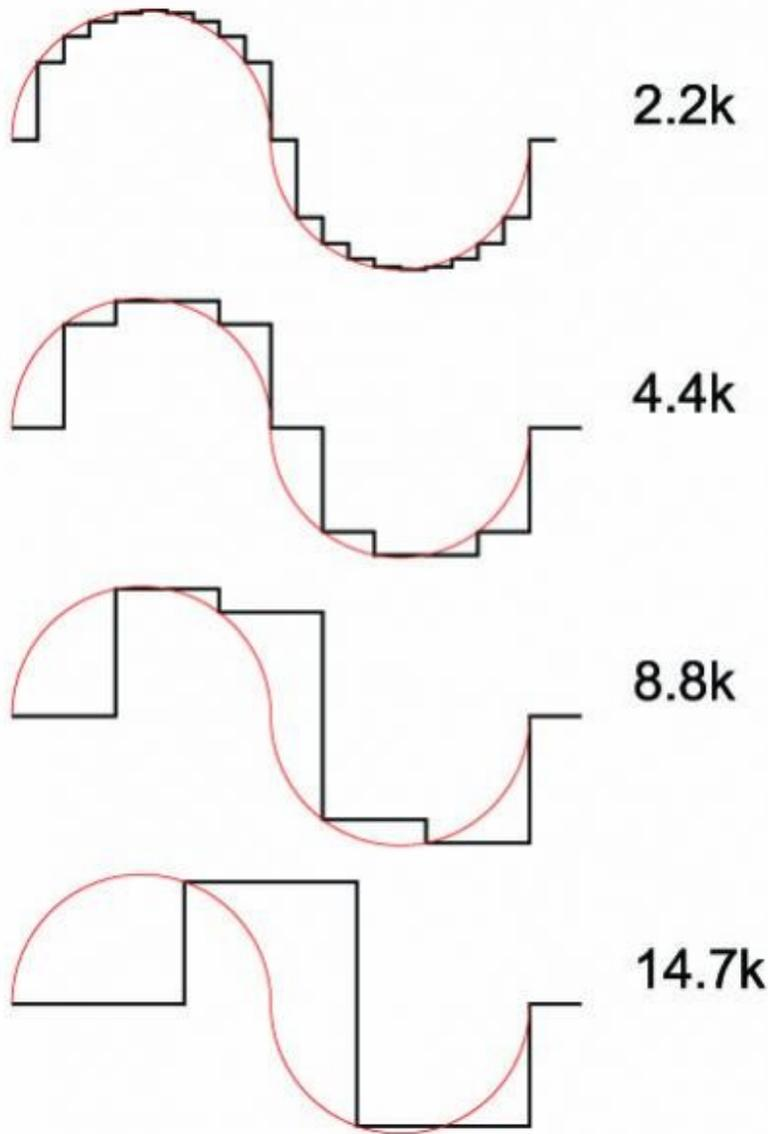
If you look at a digital approximation (black) of an analog wave (red) you can see that the right angles actually create minute increases in amplitude. Even after all the fancy algorithms of today's DSP DACS there still seems to be at minimum an echo of these hard points in the waveform.
