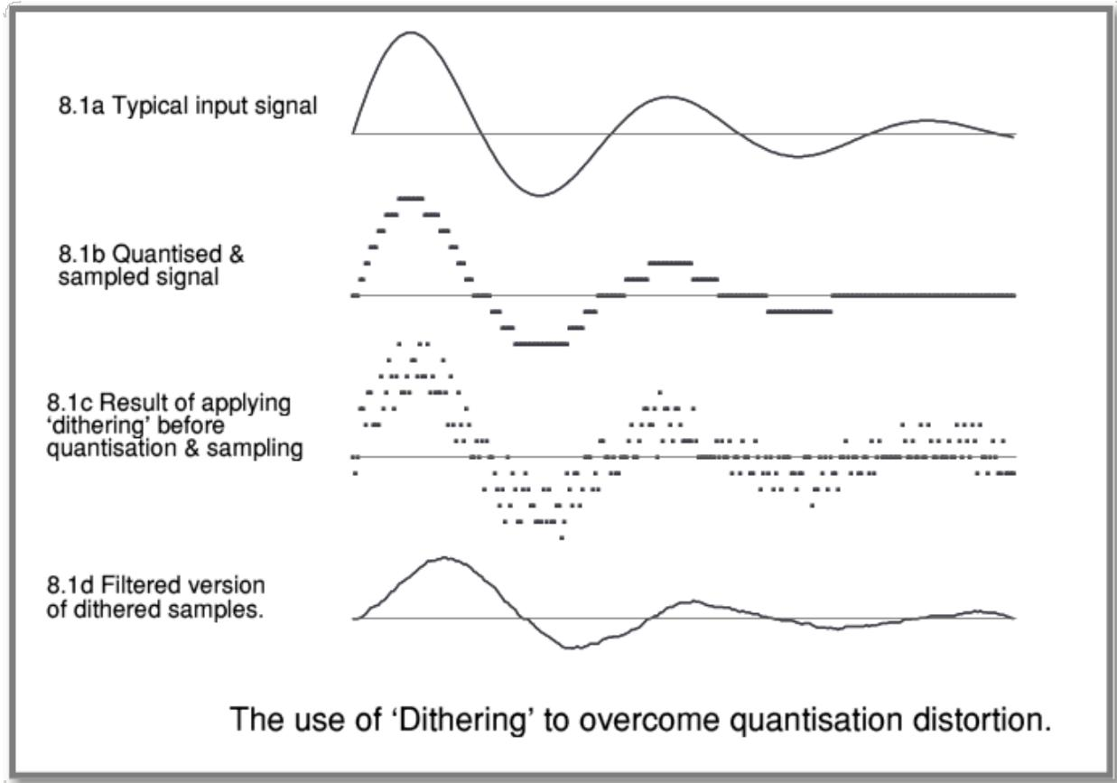
Quantization, dithering and filtering are all attempts to get a smooth continuous thread like analog. As you can see, filtering essentially glues all the dots back together and compresses them back into a fine line similar to the original input signal but with a rougher texture.
