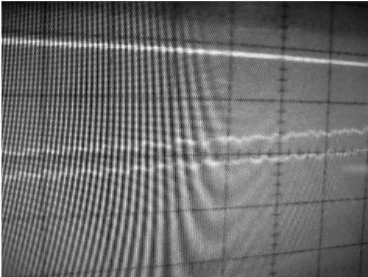
Waveform from analog function generator (top) , vs. Waveform from an Apple iPod (bottom).
