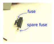
The fuse is a 3 amp, 20mm glass fuse. You can use fast or slow blow type replacements in the amp. It is located INSIDE the IEC connector. To access it, remove the power cord and take a small screwdriver to pry the little door open. It will come
