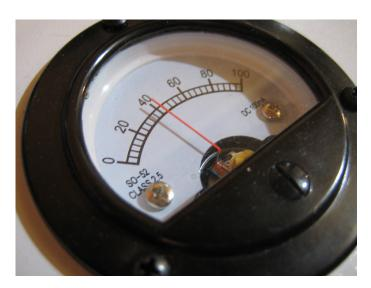
If you have perfectly matched tubes, your bias meters of which there is one for each of the two output tubes, will read the same. This is typically around 38 millivolts per side. Of course different brands of tubes may read as much as 10 millivolts higher or lower than that figure.
