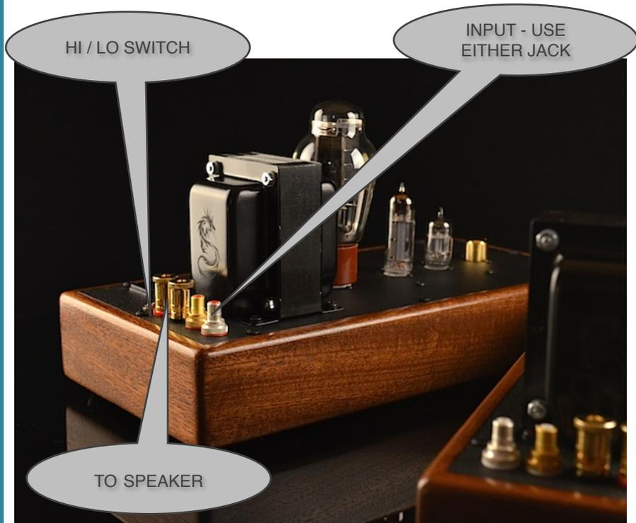
This amplifier can operate speakers as low as 2 ohms, and as high as 16 ohms and everything in-between. No harm can come to the amplifier if the speaker jacks are shorted together.
