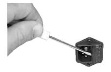
The fuse holder contains a spare fuse as shown. To reinstall just snap the new fuse in place and snap the fuse holder back into the IEC connector.
