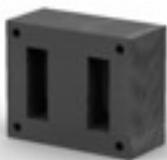
Our transformers cores (shown left) are made with M-6 29 Gauge - 0.014" (0.355 mm) Grain Orientated Electrical Transformer Steel Lamination with steam blue oxide on the surfaces and edges to minimize stray losses between laminations.
