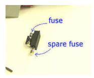
The fuse is a 3 amp, 20x5mm glass fuse. You can use fast or slow blow type replacements in this amp. It is located INSIDE the IEC connector. To access it, remove the power cord and take a small screwdriver to pry the little door open. It will come completely out of the IEC connector and not only holds the fuse, but has a spare fuse in it as well.
