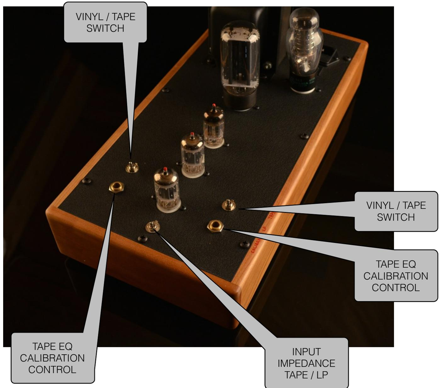
The Tape Equalization can be calibrated for each channel. The range of the calibration spans the difference between NAB and IEC curves so you can precisely calibrate the ZP3 for either one.
