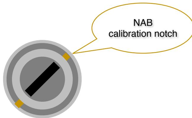
The Tape EQ calibration is an infinitely adjustable potentiometer that can also be adjusted by ear making it possible to dial in the frequency balance on a tape by tape basis. This comes in very handy for improving tapes that sound a little "off".
