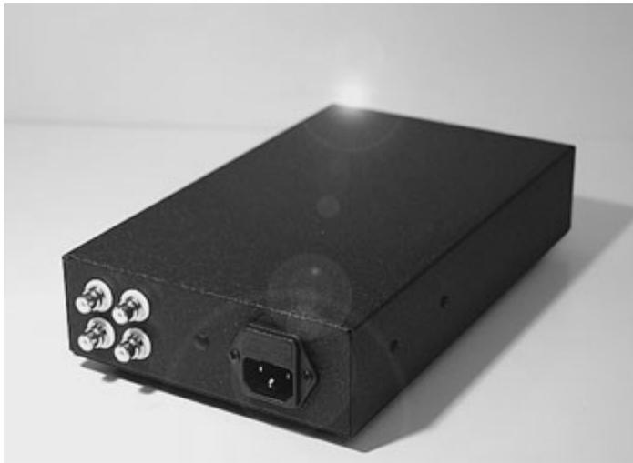
The ZOX features a IEC connector with built in fuse holder. When the power cord is removed you can access the fuse holder.
